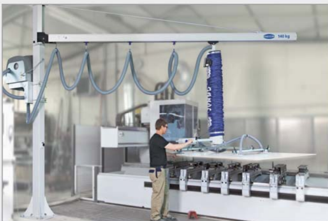
Complete handling system with vacuum tube lifter Jumbo and crane
