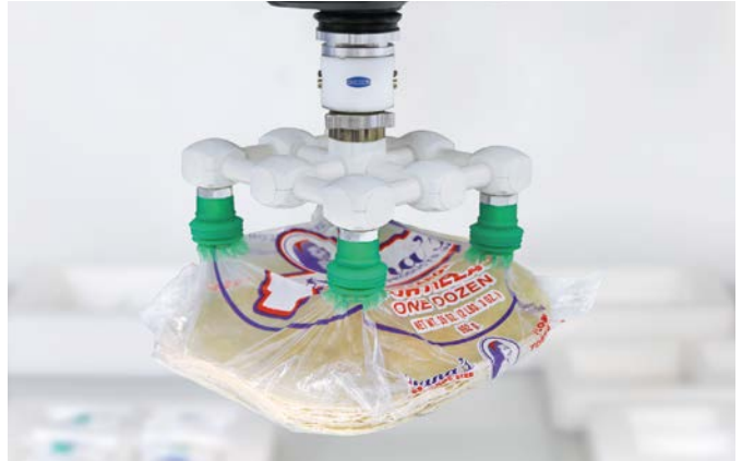
Vacuum end effector with bellows suction cups SPB4f handling pouches with many wrinkles and a low filling degree
