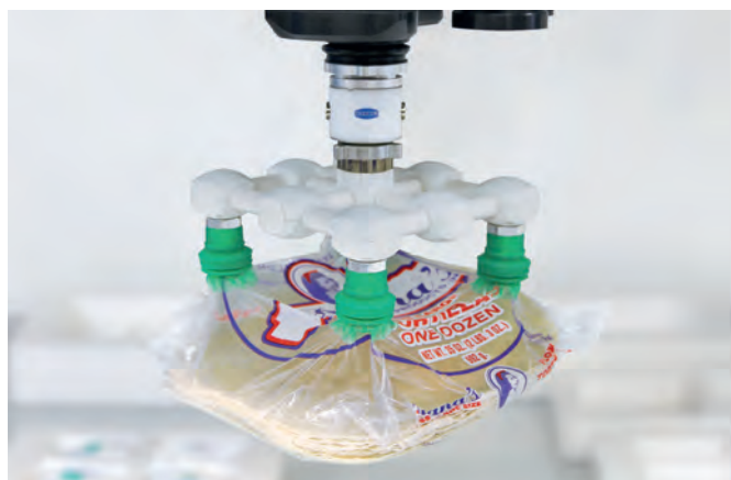
Vacuum end effector with bellows suction pads SPB4f handling pouches with many wrinkles and a low filling degree.
