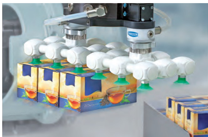
Vacuum end effector with flat suction pads SPF handling boxes of tea
