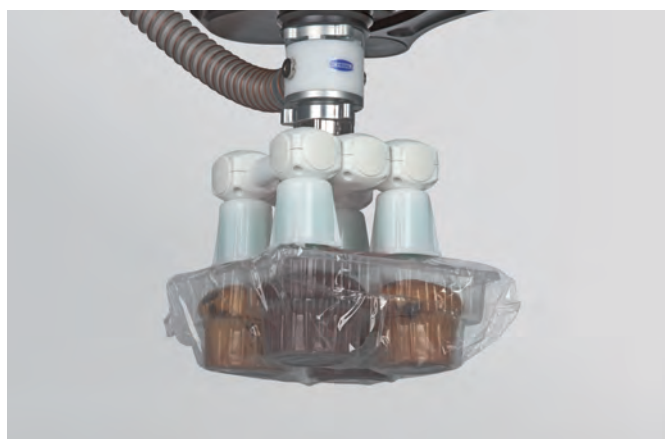
Vacuum end effector with bellows suction pads SPB4 and stabilization elements handling unstable flow-wrap packaging
